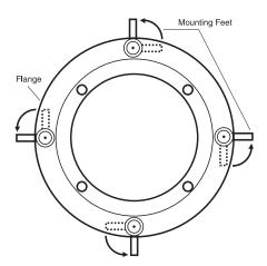
CAUTION: Over tightening may warp the baffle, crack the ceiling, cause the flange to distort, and make the grille difficult to install.
